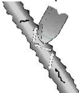
Scanning technique to detect surface or near surface cracks in the weld cap
